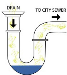
Dry or leaking drain/p-trap: Sewer gases are NOT contained
